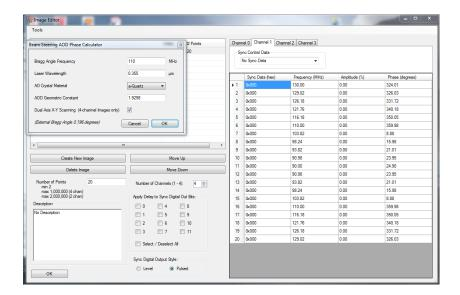
Input Bragg Angle Frequency (Usually set at the AOD centre frequency, 110MHz) Input Laser Wavelength (355nm)
